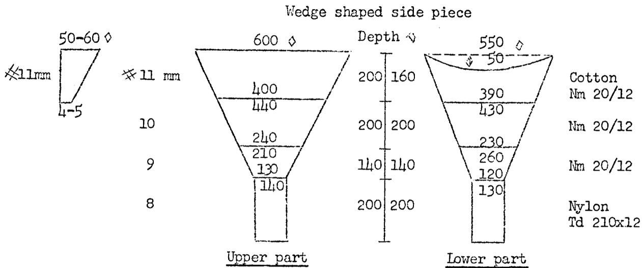
Figure 3. Construction of the net.
