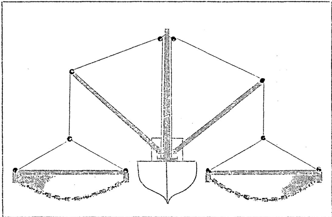
Figure 2. Scheme of a shrimp cutter with two beam trawls.
